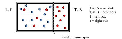
Fig 2.1 Gas A is separated from the mixture at the right box and has pressure equal to the total pressure at the left box
