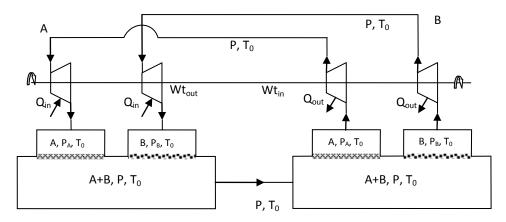
FIG 1.2 Mixing & separation of two ideal gases "reversibly" in a closed loop
