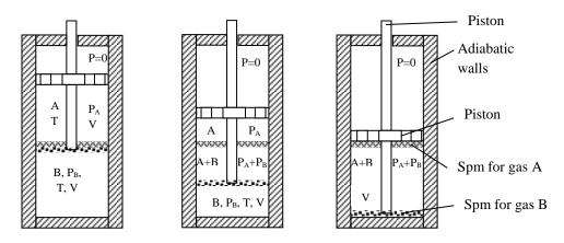
FIG 1.1 Reversible mixing of two ideal gases A and B with two semipermeable membranes
