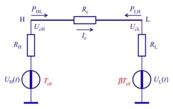
**Figure 4.** Schematic for illustrating the elimination of the Second-Law-attack and the BSY-attack by introduction of a proper temperature offset. The notation is consistent with that in Figure 1.
