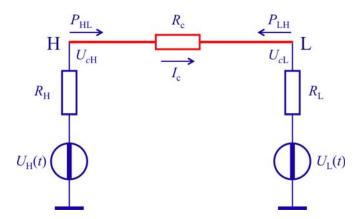
**Figure 2.** Scheme devised to illustrate the Bergou-Scheuer-Yariv attack and the Second-Law-attack. Alice's and Bob's locations are arbitrary in the figure. During the Second-Law-attack, the powers flowing out from the "H" and "L" ends of the cable are calculated and compared. The temperature of the cable resistor  $R_c$  can be neglected because of the high noise temperature of the generators. The notation is consistent with that in Figure 1.
