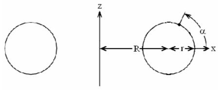
Define the inner I and outer/external/equatorial O radii of a torus
