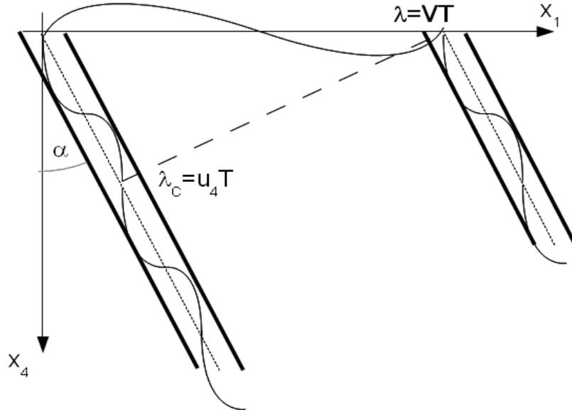
Fig.3. It is shown the vortex tube position in the time moments  $t=0$  and  $t=T$ , the period of the stream rotation around the vortex axis. One stream line into the vortex tube is outlined.
