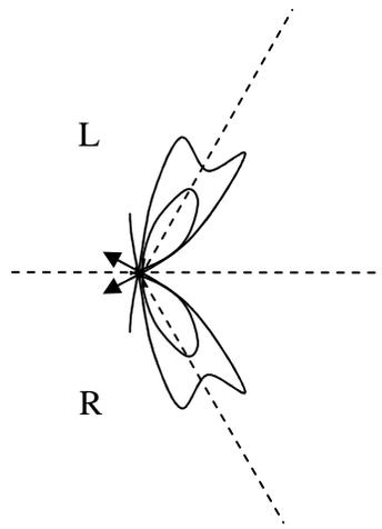
Front view of more and less bent virtual particle paths of a positively electrically charged particle propagating out of the page
