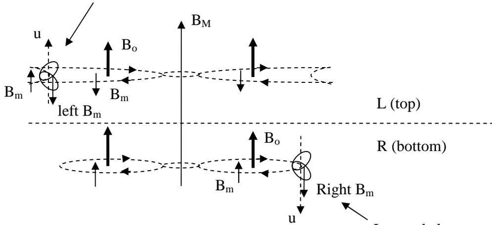
Electron at different times in more and less bent orbital portions in the (s) orbital of a hydrogen atom (shown in planes in a horizontally sectioned view).
