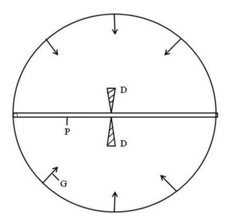
**Fig. 1.** Convergent Gudeley shock wave G onto magnetized fusion target in hollow pipe P with additional deuterium D for propagating burn into a region with an increasing diameter (horn) for a growing thermonuclear detonation wave.
