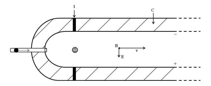
**Fig.6.** Faraday generator for chemical-nuclear energy conversion into electric energy : F hybrid chemical-fusion mini-bomb, B magnetic field directed perpendicular to plane of drawing and produced by electromagnets, v velocity of plasma fire ball which induces electric field  $\mathbf{E} = (\mathbf{v} / \mathbf{c}) \ge \mathbf{B}$ , C wall confining plasma flow, I insulator.
