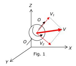
The velocity vector on two orthogonally related component is decomposable:  $V_1$  on a direction of rotation axis of a body and  $V_2$  of perpendicular this axis.
